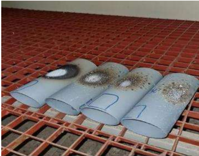
Figure 8. Samples from left to right, showing increasing boron additive content [9]
